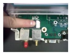
Re-secure the SIM by moving the SIM bar (to the right)
