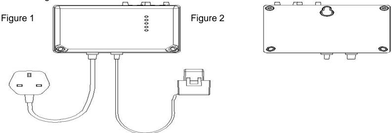
Fix the device to an appropriate position before making any electrical connections. Install one screw on the fixed surface of the intended mounting position and the hang the device on the screw using the rear mounting hole as shown in Figure 2 above.
